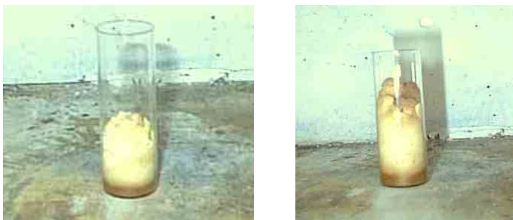
Figure 4-12 The calcium gluconate sample being foamed in the furnace at 300°C
