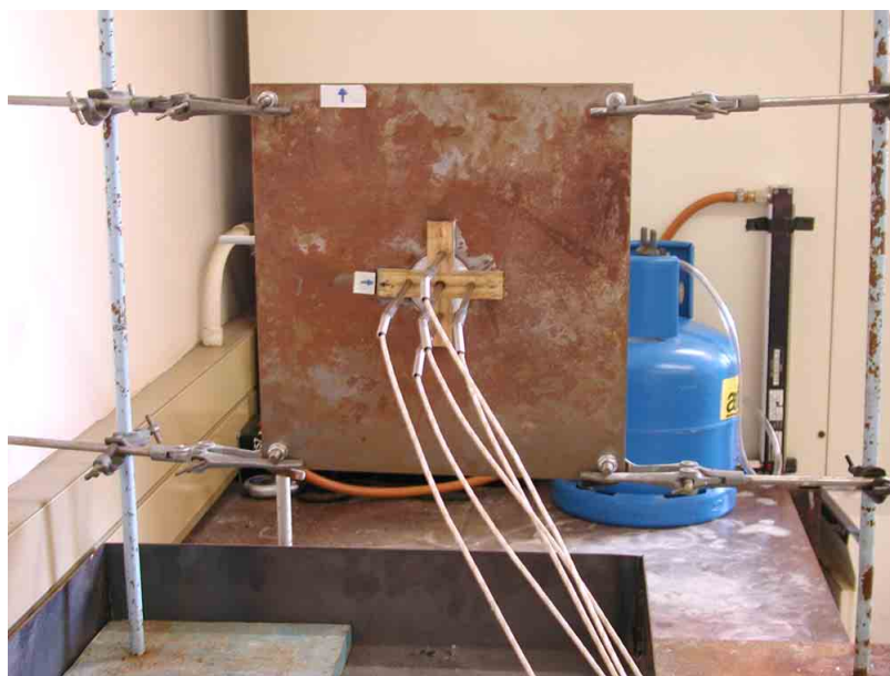
Figure 3-10 Back view of the burn test setup showing the thermocouples
