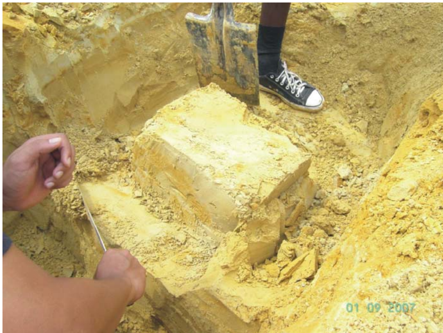
Figure 3-3. Exposing a suitable block by excavating around the block.
