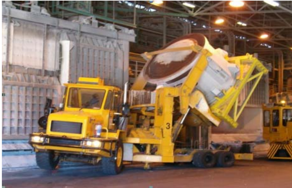
Figure 2-4 Ladle Transport Vehicle (LTV)
