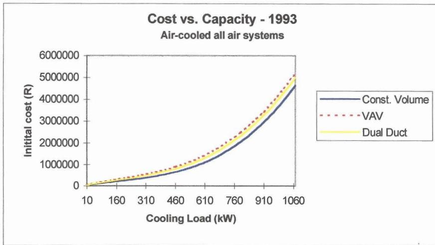
Figure 6.15 - Cost versus capacity relation for air-cooled all-air systems
