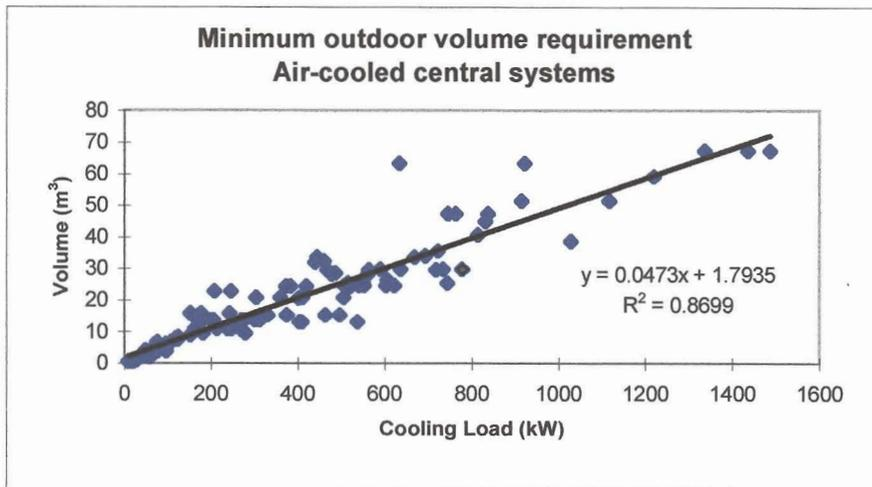
Figure 6.12 - Outdoor volume correlation for air-cooled refrigeration machines
