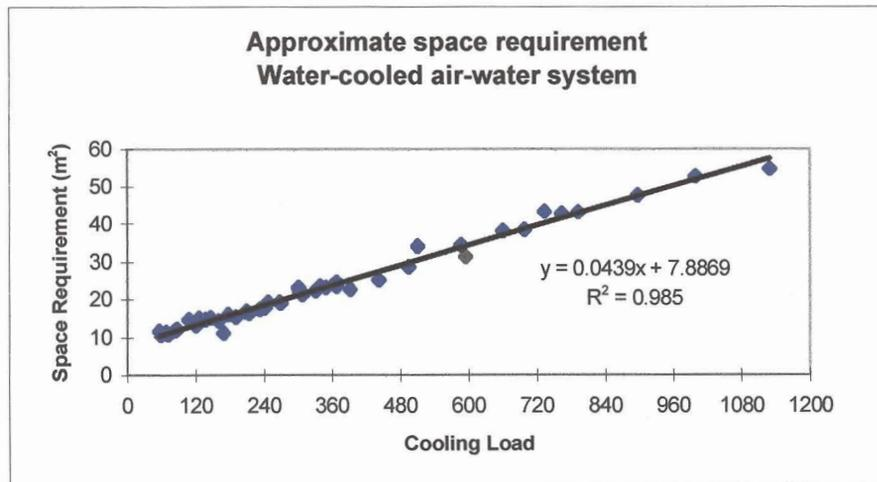
Figure 6.3 - Space requirement correlation for water-cooled air-water systems
