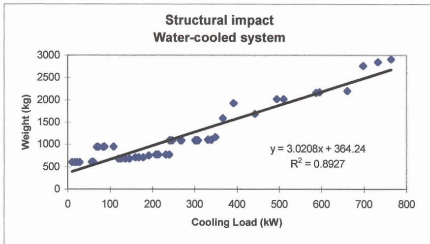
Figure 6.7 - Mass correlation for water-cooled system cooling towers
