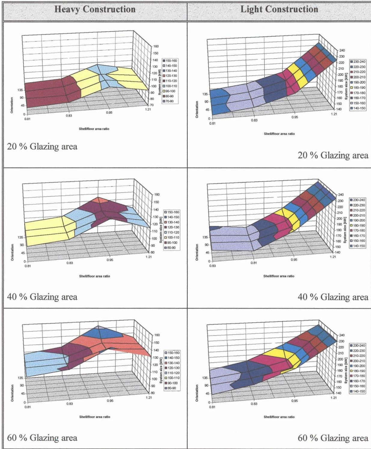
Figure 7.3 - Heating system requirements for different configurations of a 2500m<sup>2</sup> office building located in Pretoria.
