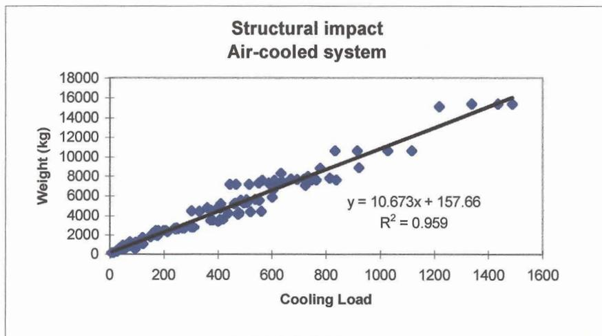
Figure 6.8 – Mass correlation for air-cooled refrigeration machine
