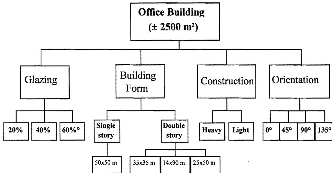
Figure 7.1 – Simulation variables used for the thermal analysis
