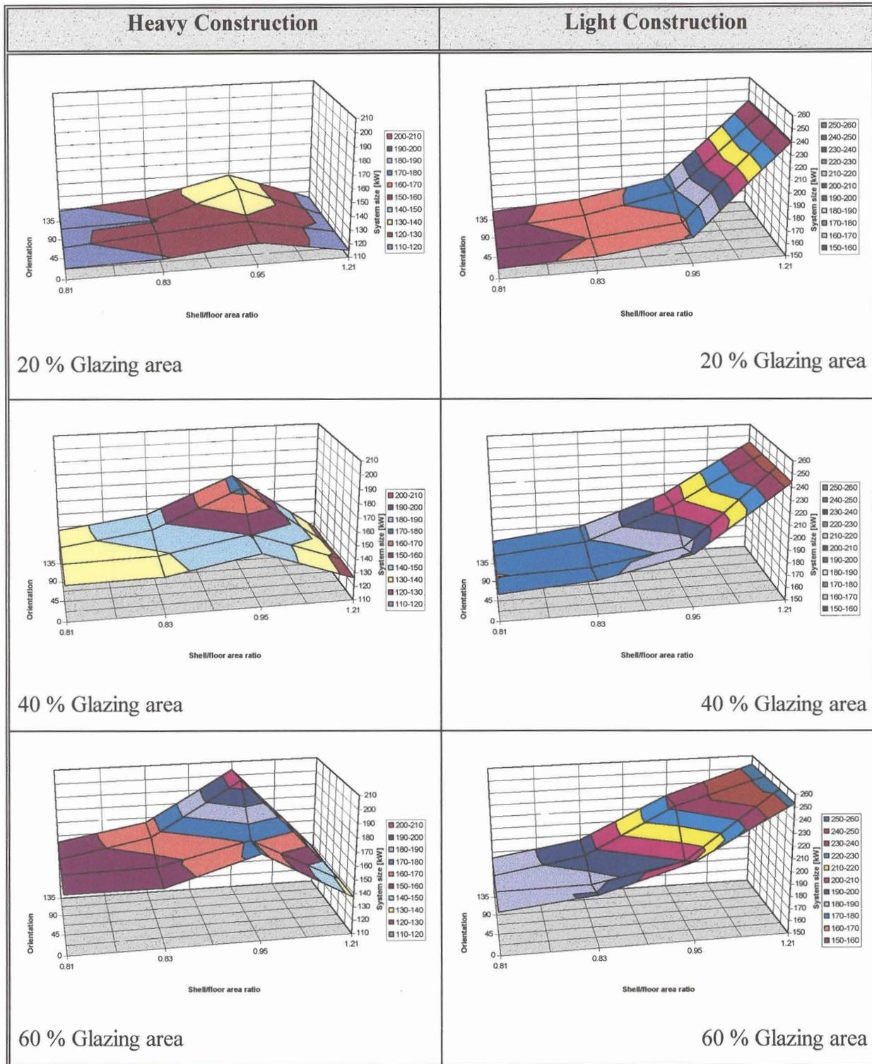
Figure 7.2 - Cooling system requirements for different configurations of a 2500m<sup>2</sup> office building located in Pretoria.
