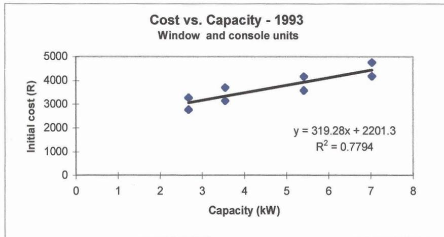
Figure 6.20 - Cost versus capacity relation for window and console units
