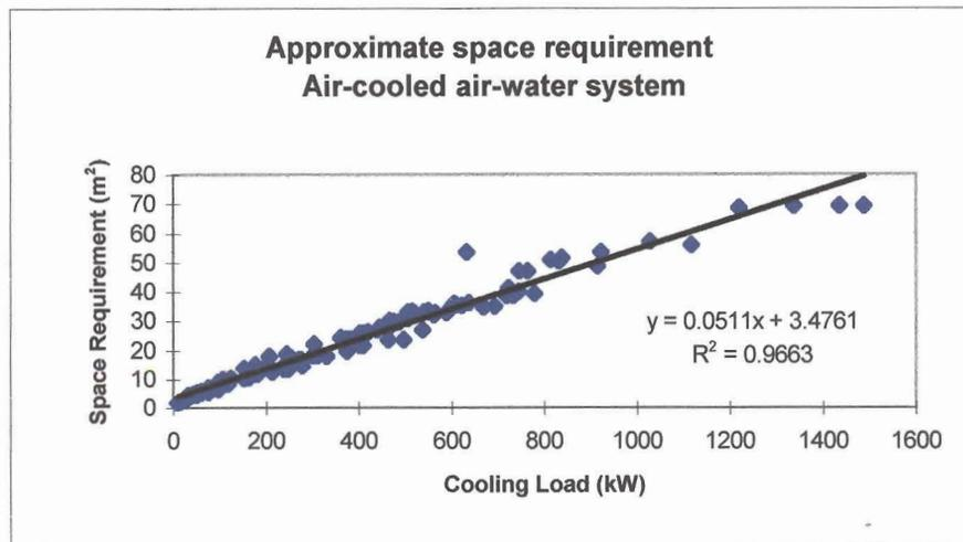
Figure 6.4 - Space requirement correlation for air-cooled air-water systems
