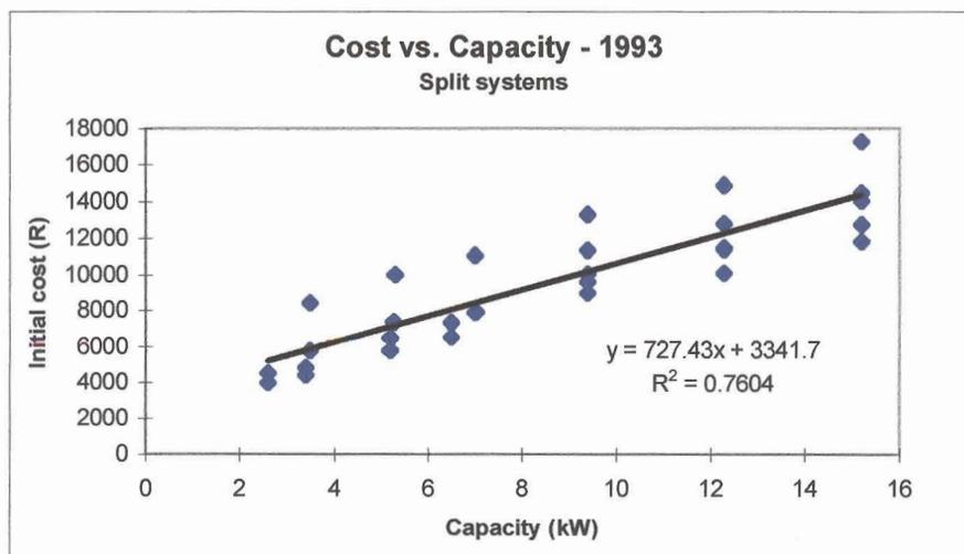
Figure 6.19 - Cost versus capacity relation for split systems
