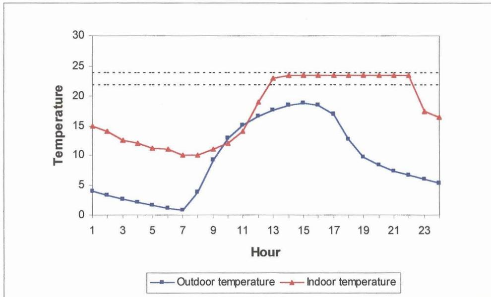
Figure 4.4 – Typical required indoor temperature profile [10].
