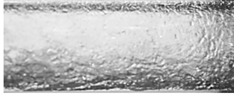
Figure 4.3: Intermittent flow - between slugs
