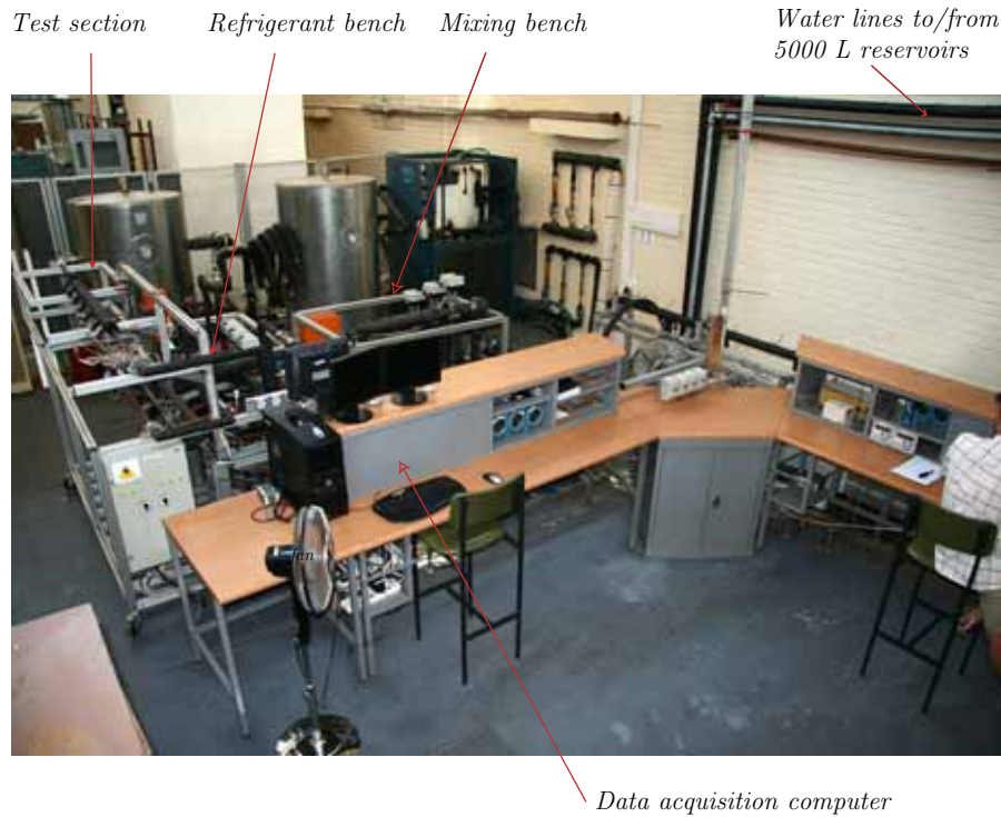
Figure 3.1: Top view of the two-phase flow experimental setup
