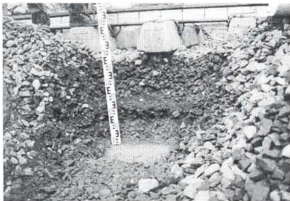
Layers above and below bitumen layer
