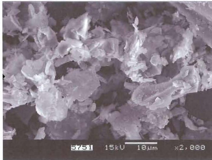
Figure 3-63: Mizpah Pond Coarse Tailings, undispersed bulk specimen.
