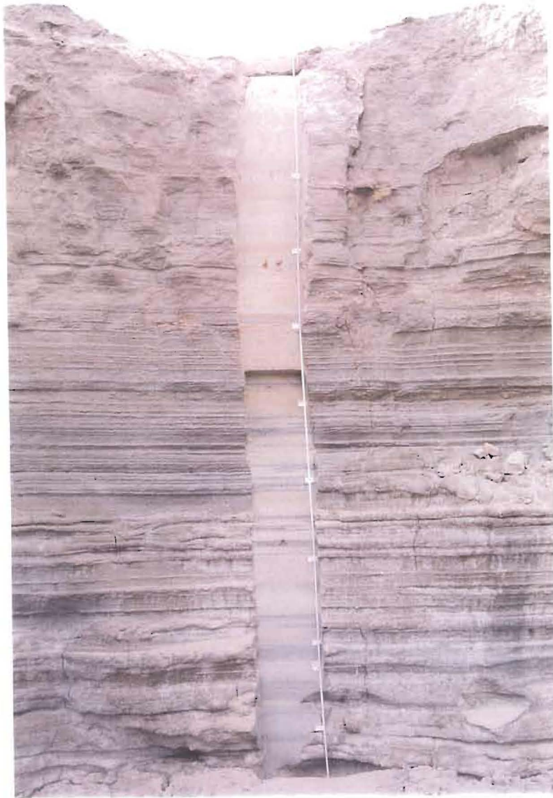
Figure 3-6: (b) Pay Dam site showing a close-up of the 5 m profile and the sampling pits.
