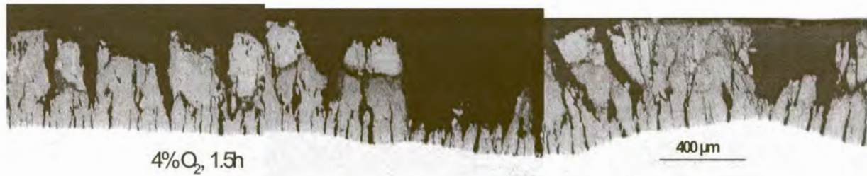
Figure 29 : Montage of descaled surface of type 412 sample (reheated at 1280 °C)
