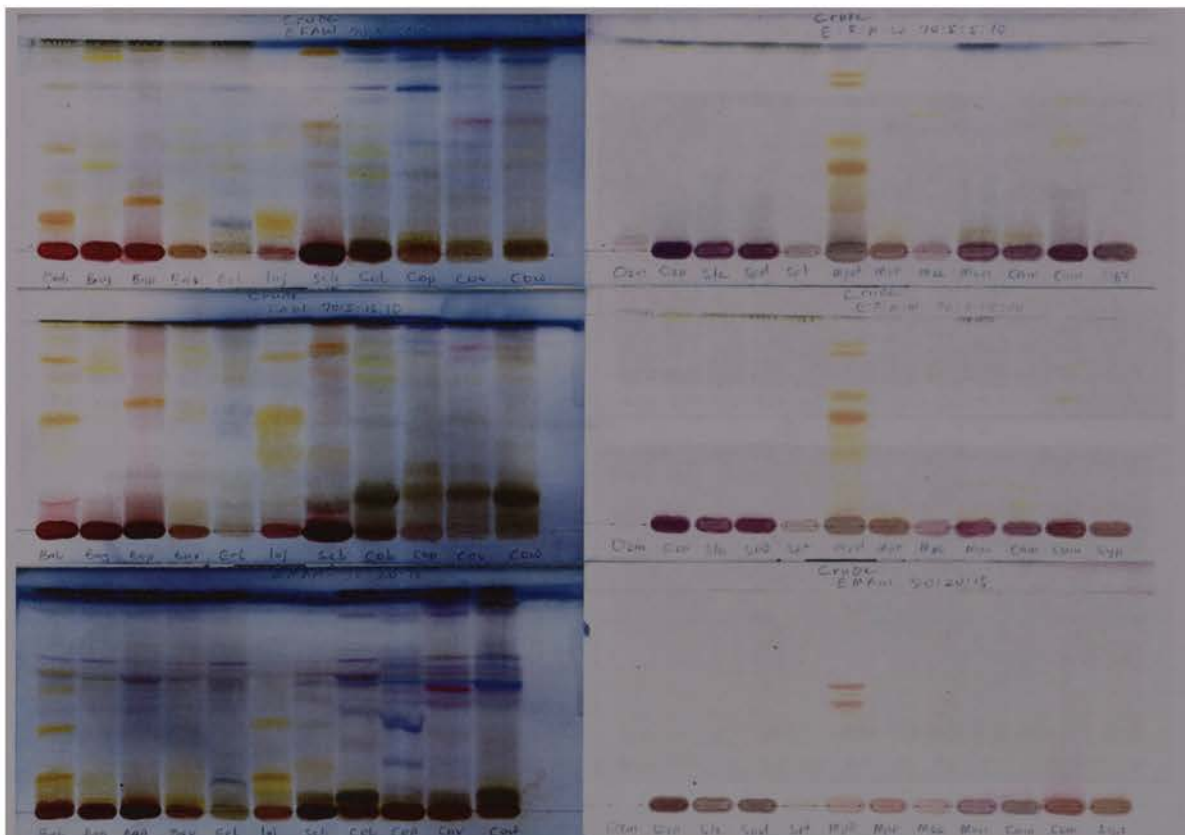
Fig.3.2. Chromatograms of 100 µg of crude extracts of different plant species developed with ethyl acetate: acetic acid: formic acid: water (75:5:5:10) (top), ethyl acetate: acetic acid: formic acid: water (70:5:15:10) (middle) and ethyl acetate: methanol: ammonia (90:20:15) (bottom) and visualized with vanillin sulphuric acid. For identity of plant species see under section 3.7.2 or under abbreviations used.
