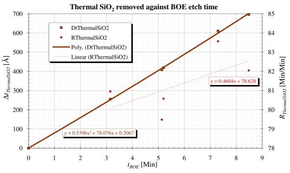
Figure D.4. Measured BOE etch rates of thermal SiO<sub>2</sub>.
