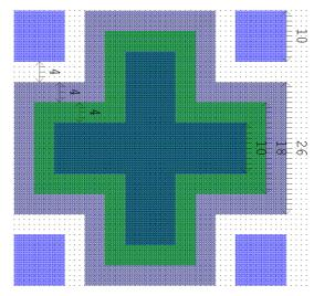
Figure 4.23. *AlignmentMarkerPhotoNoOx* layout.
