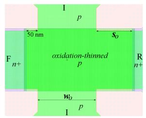
Figure 4.7. Opposite-injection SOI element layout dimension definitions.
