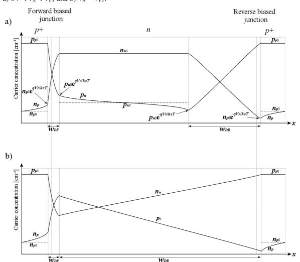
Figure 2.10 shows the electron  $(n_{xy})$  and hole  $(p_{xy})$  carrier distributions in the  $p^+np^+$  device for a)  $0V < V_A < V_{PT}$  and b)  $V_A = V_{PT}$ .
