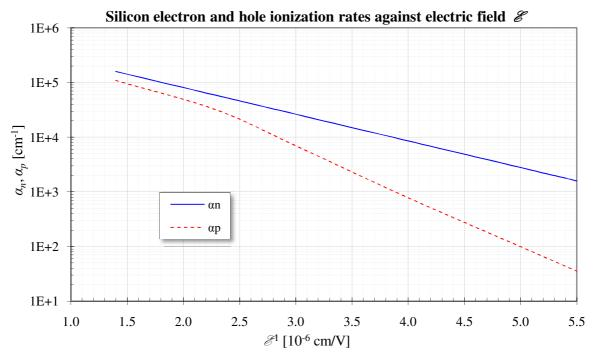
Figure 2.4. Silicon electron and hole ionization rates against electric field.
