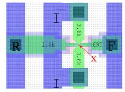
Figure 4.8. Single opposite-injector element layout on a 1-µm grid.
