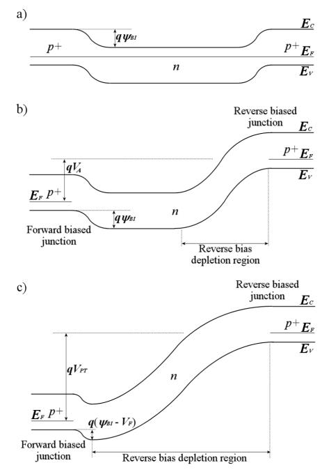
Figure 2.9. Energy-bands of the  $p^+np^+$  junctions at a)  $V_A = 0$  V, b) 0 V <  $V_A$  <  $V_{PT}$  and c)  $V_A = V_{PT}$ .
