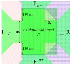
Figure 4.11. Side-injection SOI device layout dimension definitions.
