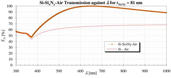
Figure 5.16. Si-Si<sub>x</sub>N<sub>y</sub>-air transmission at  $t_{SixNy} = 81$  nm.
