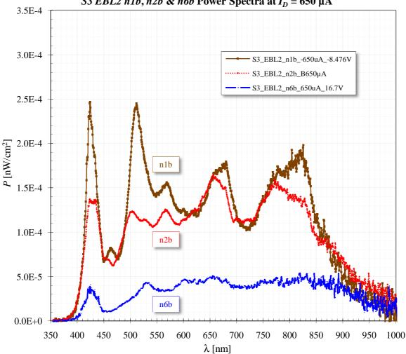
S3 EBL2 n1b, n2b & n6b Power Spectra at  $I_D = 650 \mu A$
