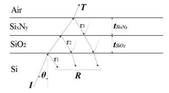
Figure 2.22. Light transmission through the Si, SiO<sub>2</sub>, Si<sub>x</sub>N<sub>y</sub> and air layer stack.
