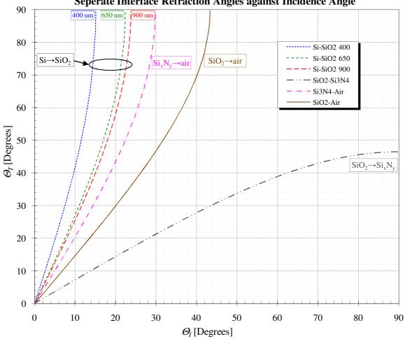
Seperate Interface Refraction Angles against Incidence Angle
