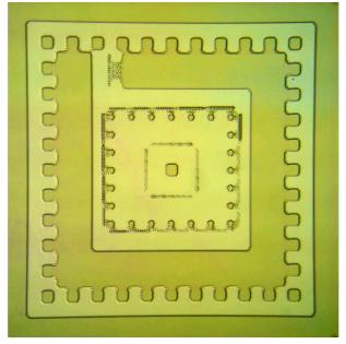
Figure 5.2. Bad Chip1 Si Island exposure (step 3f).
