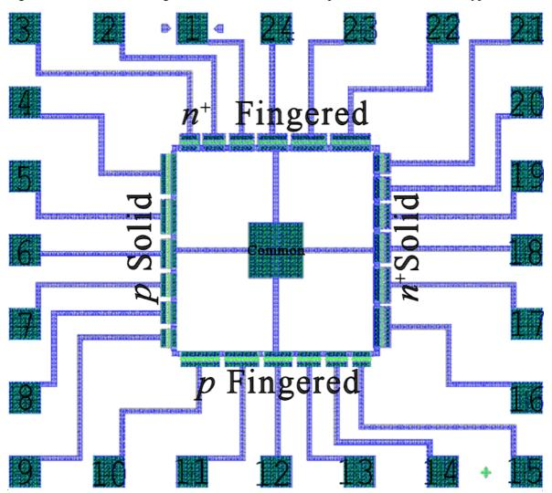
Figure 4.20 shows the configuration of the four different process-monitor resistor types.
