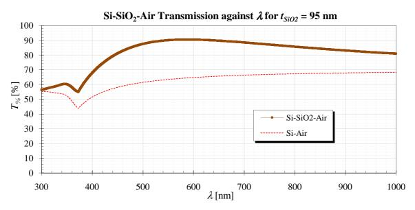
Figure 5.24. Si-SiO<sub>2</sub>-Air transmission at  $t_{SiO2} = 95$  nm.
