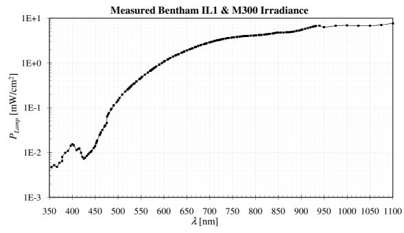
Figure B.1. Measured Bentham IL1 lamp and M300 monochromator output spectral irradiance.
