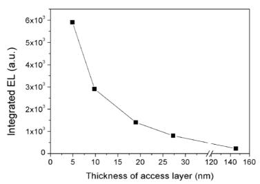
Figure 1.2 Integrated EL intensity against access layer thickness [48].
