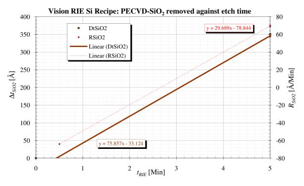
Figure D.9. Measured PECVD-SiO<sub>2</sub> etch rate in Vision Oxide RIE Si recipe.
