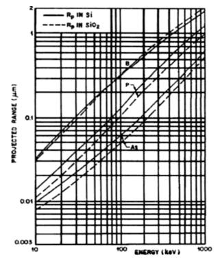
Figure 5.5. Projected ion implantation range  $Rp_{As\_SiO2}$  in SiO<sub>2</sub> [91].
