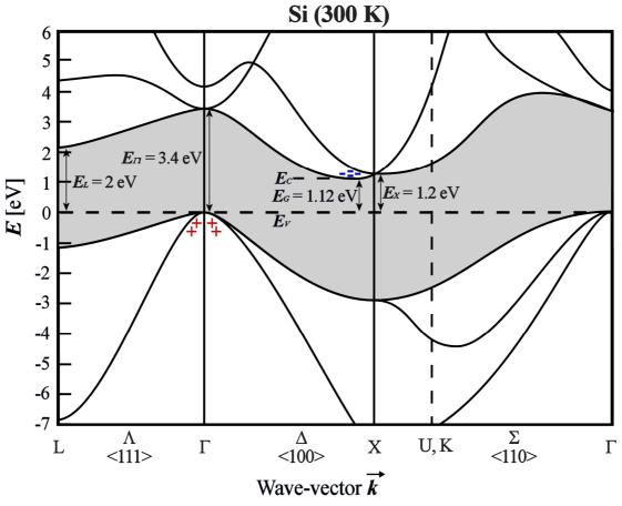
Figure 2.3. Energy band structure of Si at 300 K.
