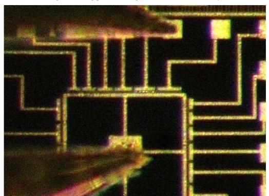
Figure 6.5 shows the light-emitting punch-through device n2b at  $I_D = 650 \mu A$ .
