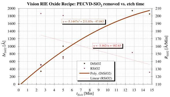
Figure D.14. Measured PECVD-SiO<sub>2</sub> etch rate in Vision Oxide RIE standard oxide recipe.
