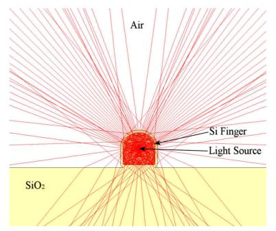
Figure 3.2. SOI finger spatial light radiation pattern simulation.
