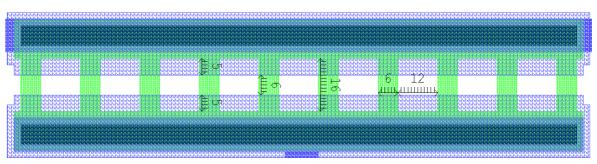
Figure 4.16. *INSiAVA1*  $n^+pn^+$  punch-through device layout.
