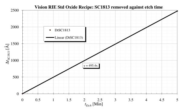
Figure D.17. Measured SC1813 etch rate in Vision Oxide RIE standard oxide recipe.
