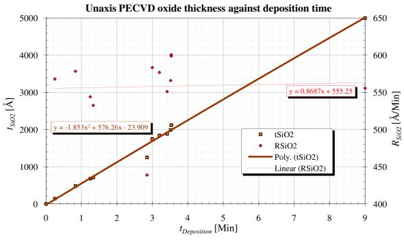
Figure D.6. Measured Unaxis PECVD SiO<sub>2</sub> deposition rates.
