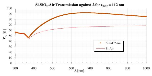
Figure 5.23. Si-SiO<sub>2</sub>-Air transmission at  $t_{SiO2} = 112$  nm.
