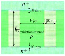
Figure 4.4.  $n^+pn^+$  punch-through finger layout dimension definitions.
