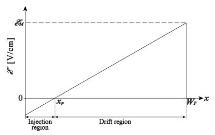
Figure 2.11. Electric field distribution in the punch-through device.
