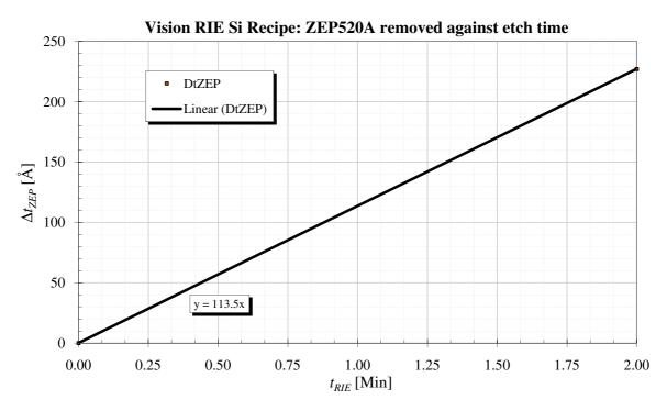
Figure D.12. Measured ZEP520A etch rate in Vision Oxide RIE Si recipe.
