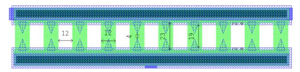
Figure 4.17. *INSiAVA1* triangular  $n^+pn^+$  punch-through device layout.
