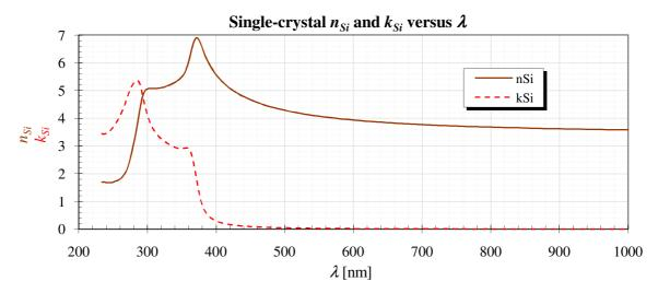
Figure 2.15 plots silicon's refractive index and extinction coefficient against wavelength.
