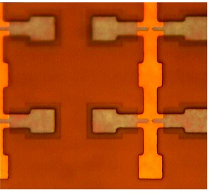
Figure 5.8. Arsenic EBL pattern before implant (step 4h).
