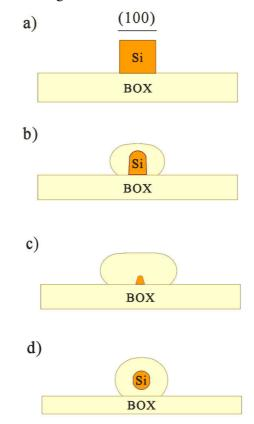
Figure 2.30. Si shape a) before oxidation, during b), c) continuous and d) undercutting oxidation.
