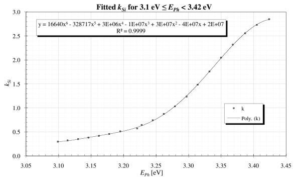
Figure 2.19. Silicon extinction coefficient  $k_{Si}$  polynomial fit for 3.1 eV  $\leq E_{Ph} < 3.42$  eV.
