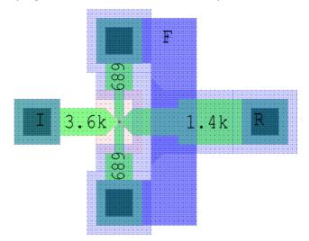
Figure 4.12. Single side-injection SOI injector element layout on a 1-µm grid.
