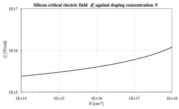
Figure 2.5. Si critical electric field  $\mathscr{E}_{c}$  against background doping N.
