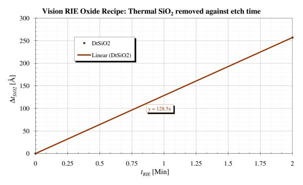
Figure D.15. Measured Thermal SiO<sub>2</sub> etch rate in Vision Oxide RIE standard oxide recipe.
