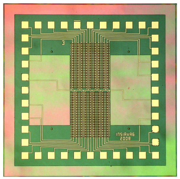
Figure 5.28. Micro-photograph of finalized *Chip3*.
