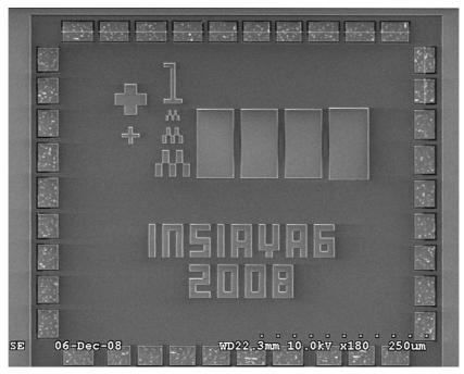
Figure 5.19. Chip2 after oxidation EBL de-scum (step 6k).
