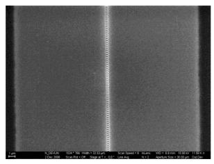
Figure 5.10. EBL finger spacing pattern (step 5a).
