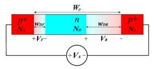
Figure 2.8. Punch-through voltage variable definitions.
