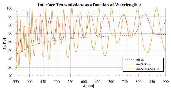
Figure 2.24. Comparison of Air-Si<sub>x</sub>N<sub>y</sub>-SiO<sub>2</sub>-Si, Air-SiO<sub>2</sub>-Si and Air-Si transmissions.
