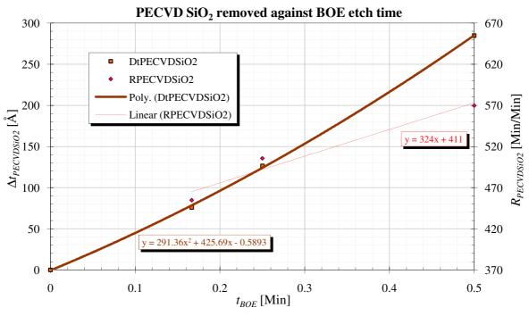
Figure D.5. Measured BOE etch rates of PECVD SiO<sub>2</sub>.
