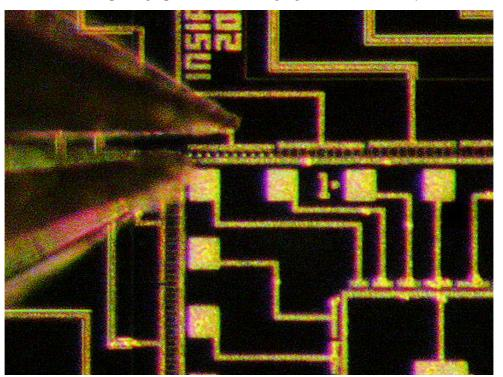
Figure 6.3. Electrical probing of test-device *D3b*.
