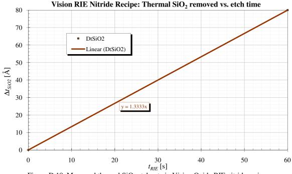
Figure D.19. Measured thermal SiO<sub>2</sub> etch rate in Vision Oxide RIE nitride recipe.
