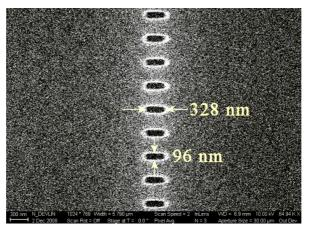
Figure 5.11. EBL finger spacing detail (step 5a).
