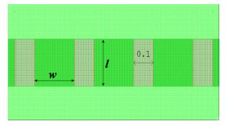
Figure 4.18. Process monitor resistor finger dimension definition.
