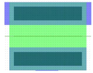
Figure 4.19 shows a 100-finger process monitoring resistor device layout.
