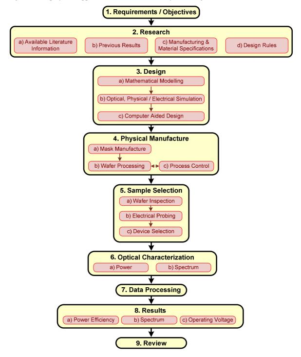
Figure 1.4. Activity flow diagram.
