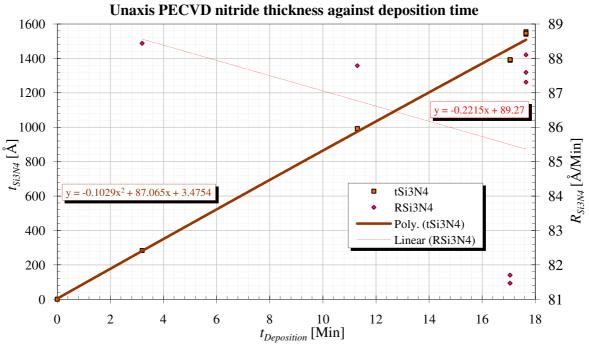
Figure D.7. Measured Unaxis PECVD Si<sub>x</sub>N<sub>y</sub> deposition rates.
