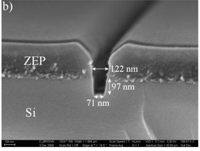
Figure 5.14. 100 nm ICP groove etch test.
