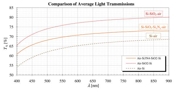
Figure 2.25. Average light transmissions through Si-air, Si-SiO<sub>2</sub>-air and Si-SiO<sub>2</sub>-Si<sub>x</sub>N<sub>y</sub>-air stacks. As shown in above plot, the simple Si-air interface (without SiO<sub>2</sub> and Si<sub>x</sub>N<sub>y</sub> layers), while eliminating the interference patterns in Figure 2.24, also results in the lowest average light power exiting into the air above the chip.
