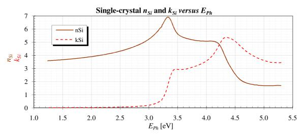
Figure 2.16. Silicon refractive index  $n_{Si}$  and extinction coefficient  $k_{Si}$  against photon energy  $E_{Ph}$ .
