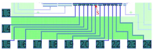
Figure 4.3. Finger junction devices layout.
