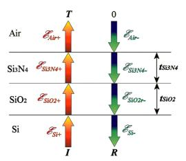
Figure 2.23. Electromagnetic fields in the Si-SiO<sub>2</sub>-Si<sub>x</sub>N<sub>y</sub>-air interfaces.
