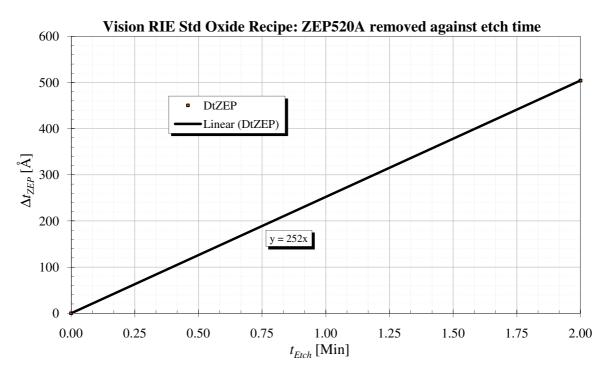
Figure D.18. Measured ZEP520A etch rate in Vision Oxide RIE standard oxide recipe.
