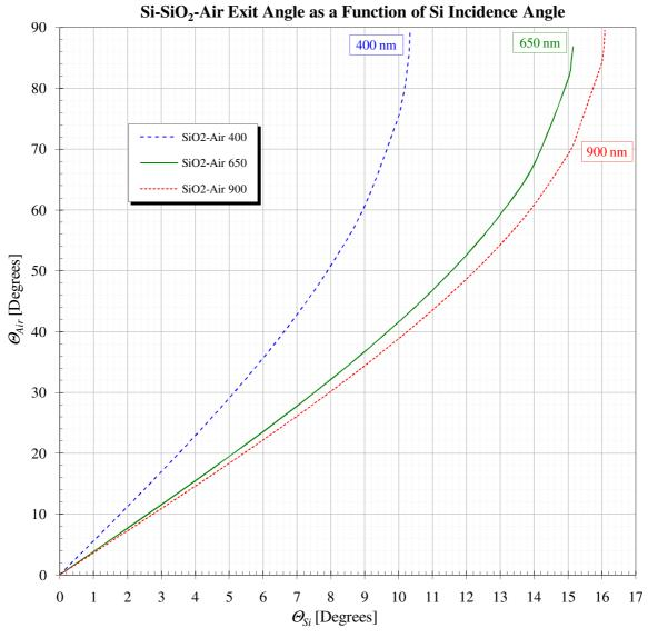
Figure 2.28. Single interface transmission angles against incidence angle.
