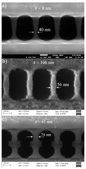
Figure 5.25. a), b) avalanche and c) punch-through SOI finger dimensions after thinning oxidation. The Si finger thicknesses indicated in above images are estimates interpolated from reflective spectrometer measurements of the oxidation monitor islands. In contrast to the broad, but thin fingers in Figure 5.25 a), the fingers in Figure 5.25 b) are more thick than narrow.
