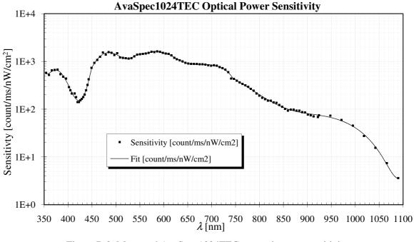
Figure B.2. Measured AvaSpec1024TEC spectral power sensitivity.
