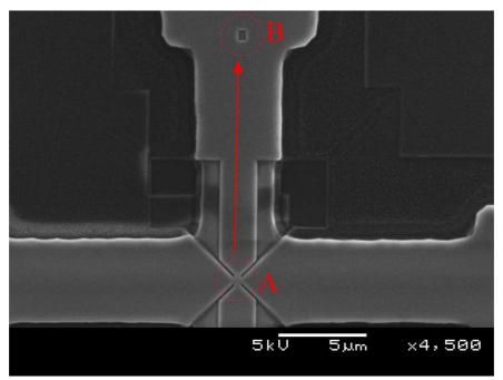
Figure 5.22. EBL oxidation window 50  $\mu$ m vertical shift.
