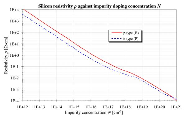
Figure 2.1. Silicon resistivity as a function of impurity doping concentration.
