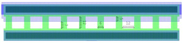
Figure 4.14. INSiAVA1  $n^+p$  avalanche breakdown device layout.
