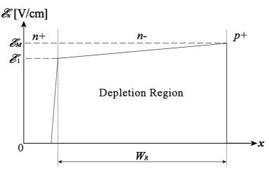
Figure 2.12. Electric field distribution in a reach-through device.
