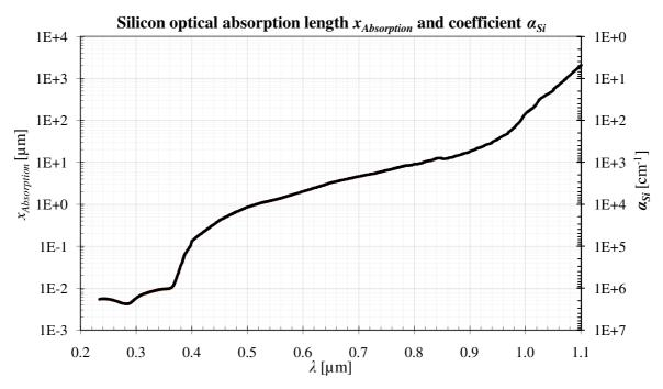
Figure 2.21. Silicon optical absorption distance  $x_{Absorption}$  and coefficient  $\alpha_{Si}$  against wavelength  $\lambda$ . Figure 2.21 illustrates how 63 % of light with  $\lambda = 350 \,\mu\text{m}$  is absorbed within 10 nm of silicon, but light with  $\lambda = 1 \,\mu\text{m}$  can travel more than 100  $\mu\text{m}$  through silicon.
