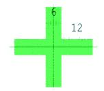
Figure 4.21. *AlignmentMarkerEBL* layout.
