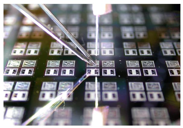
Figure 6.7. Spectroscopic probing of the SOI light-sources.
