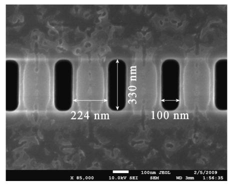
Figure 5.20. Oxidation window opening over the approximately 117 nm thick Si fingers.
