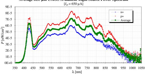
Average 0.35 µm CMOS Avalanche Light Source Power Spectrum
