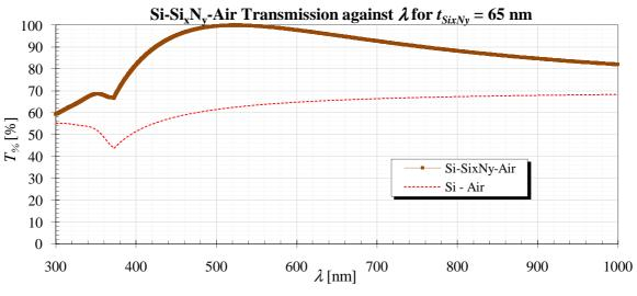
Figure 5.17. Si-Si<sub>x</sub>N<sub>y</sub>-air transmission at  $t_{SixNy} = 65$  nm.
