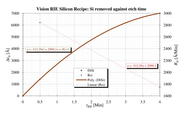
Figure D.8. Measured Si etch rate in Vision Oxide RIE Si recipe.
