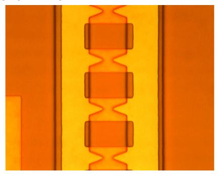
Figure 5.9. After Arsenic Photo RIE (step 4m).
