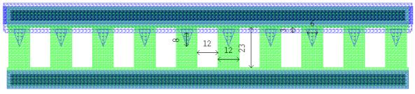
Figure 4.15. Triangular *INSiAVA1*  $n^+p$  avalanche breakdown device layout.
