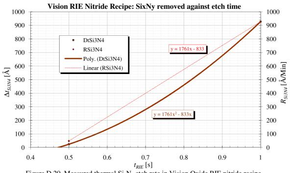
Figure D.20. Measured thermal  $Si_xN_y$  etch rate in Vision Oxide RIE nitride recipe.
