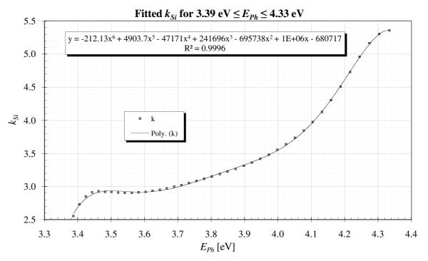
Figure 2.20. Silicon extinction coefficient  $k_{Si}$  polynomial fit for 3.39 eV  $\leq E_{Ph} \leq 4.33$  eV.
