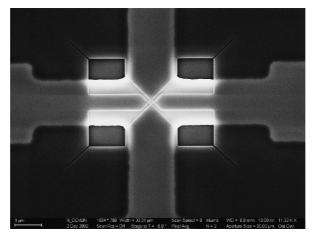
Figure 5.12. EBL injector spacing definition (step 5a).
