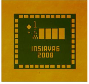
Figure 5.3. Proper Chip2 Si Island exposure (step 3f).
