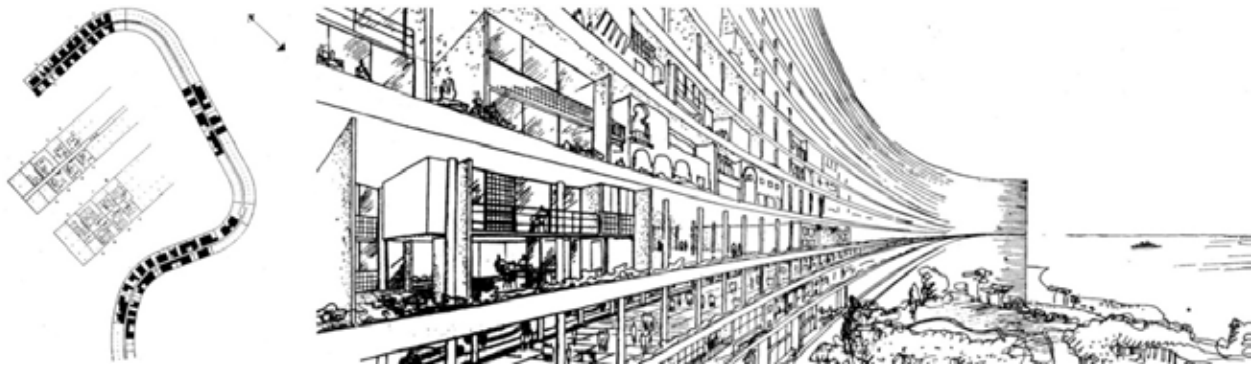
Figure 12 A close-up view of the 23-storey apartments underneath the elevated roadway (source: Le Corbusier 1964: 247).
