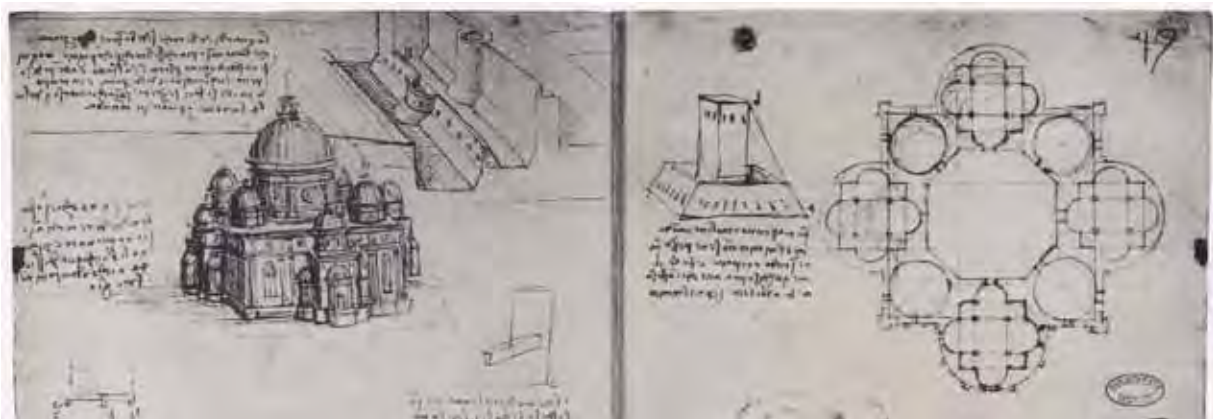
Figure 21 Leonardo da Vinci, sketches of plans and elevations of a domed church with the central space and eight domed side chapels based on an octagonal pattern extended by eight smaller domes, pen, ink and black chalk, manuscript B, folio 18 recto (source: Chierici 1956: 236).
