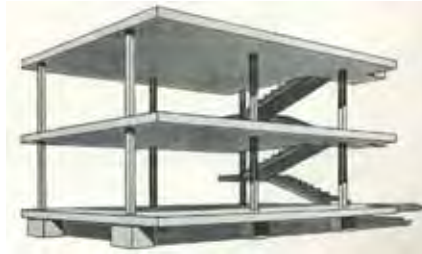
Figure 6. The Piloti system (Le Corbusier & Jeanneret, 1943: 23).
