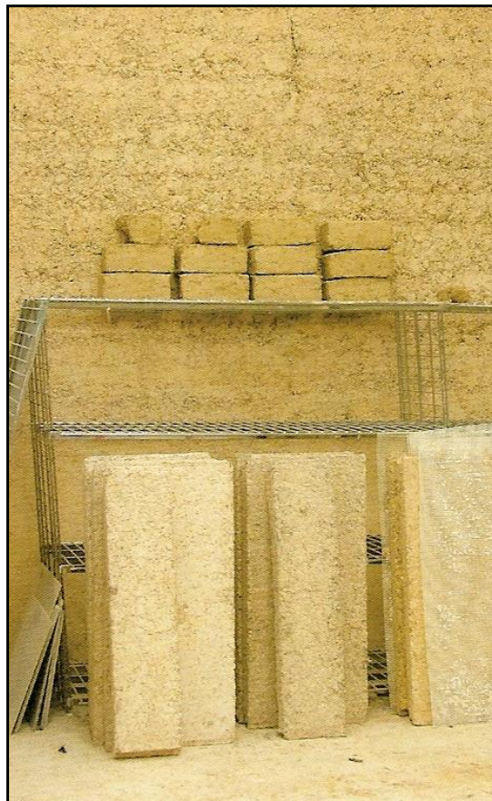
Figure 15: Precast hemp bricks and blocks made from a mould. (Allin 2005: 82)
