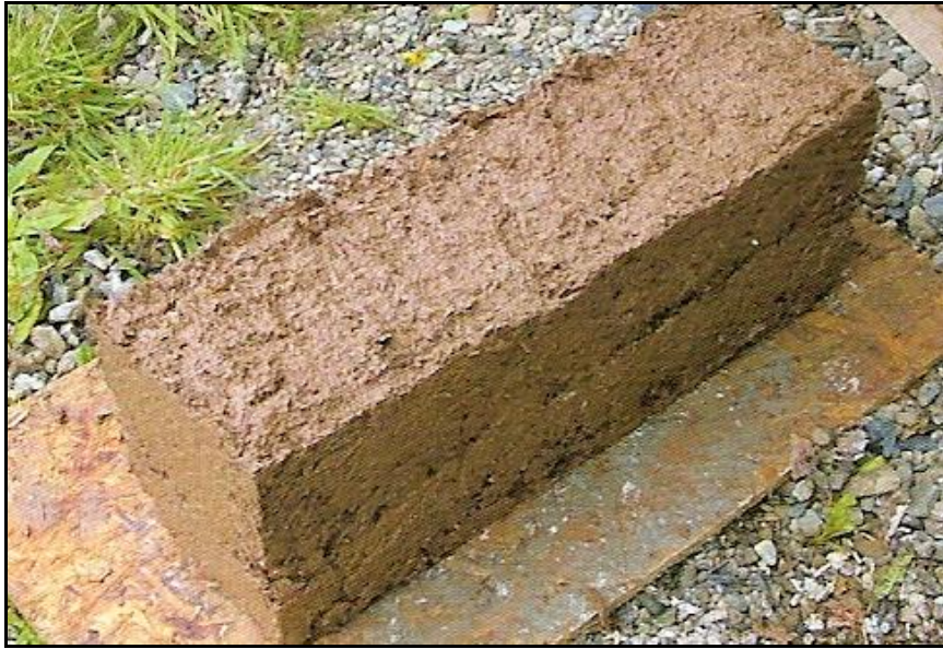
Figure 16: Precast hemp brick made from a mould. (Allin 2005: 82)
