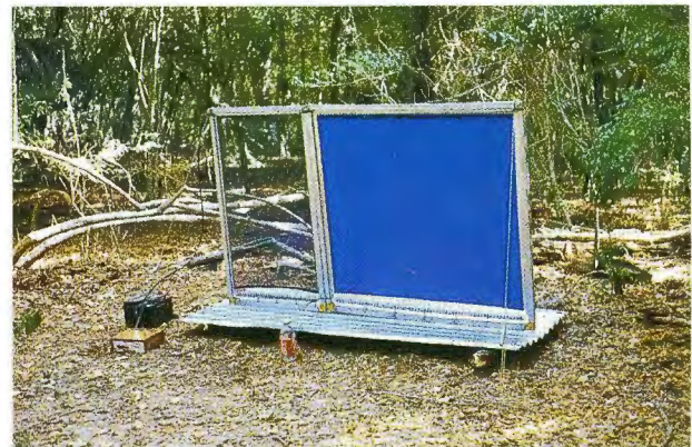
FIG. 1A Electrified grids consisting of a visual 1 x 1 m pthalogen blue (p.blue) and non-visual 0,5 x 1 m net incorporated to form a flanked (p.blue/net) target
