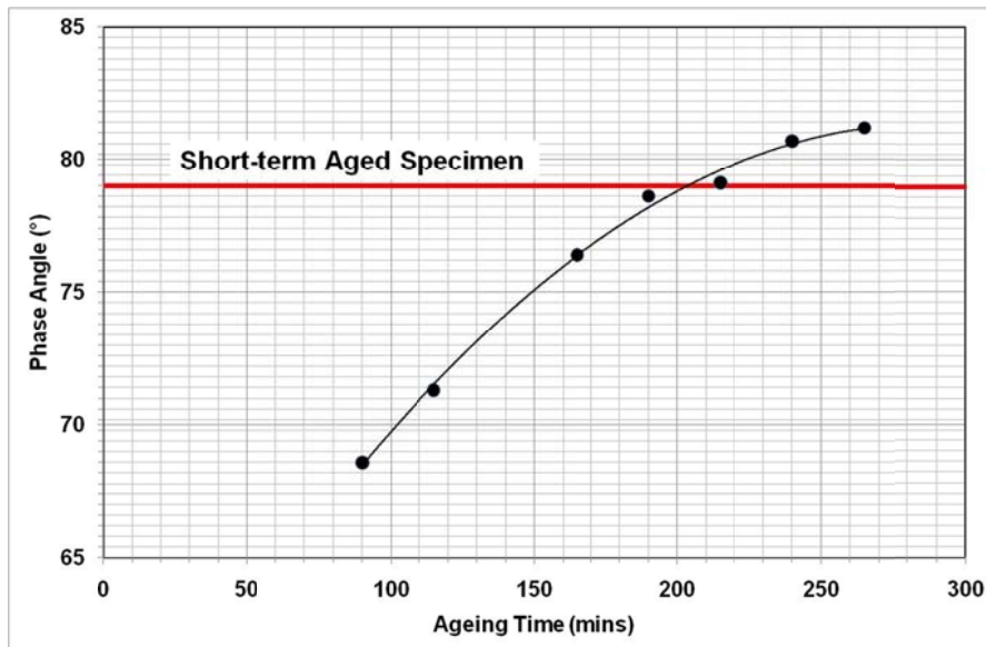
Figure 10: Phase angle, \delta (at 0.0126Hz / 70°C) vs. ageing time for an SBS modified binder sample.
