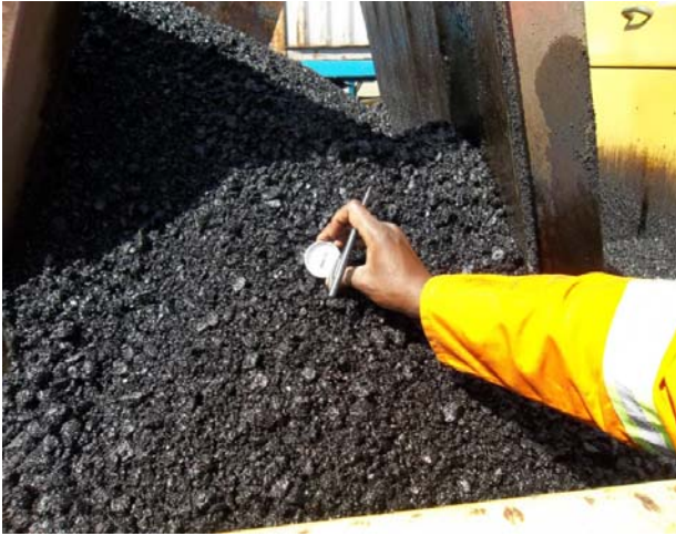
Figure 6: Mix temperature before the paver
