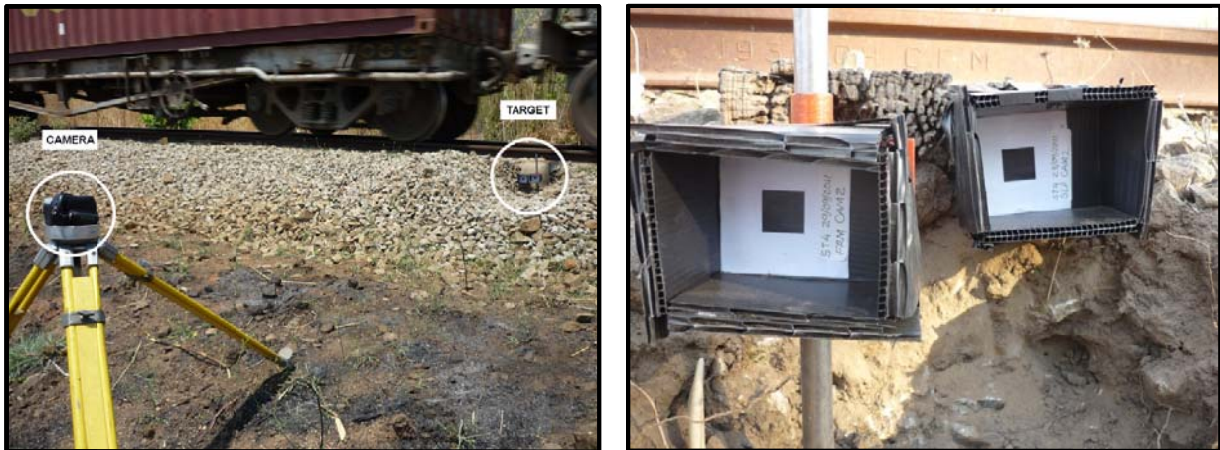
Figure 2: The RVM system comprising video camera and targets on the track structure (left) and a close up of the targets fixed to a formation reference rod and a wooden sleeper (right).
