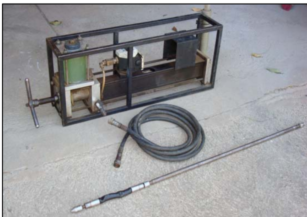
Figure 1: The Pencil pressuremeter with water reservoir, pressure chamber and probe (left) and a photo of a typical test pit where the whole for insertion of the probe is being drilled (right)
