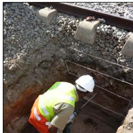
Figure 1: The Pencil pressuremeter with water reservoir, pressure chamber and probe (left) and a photo of a typical test pit where the whole for insertion of the probe is being drilled (right)
