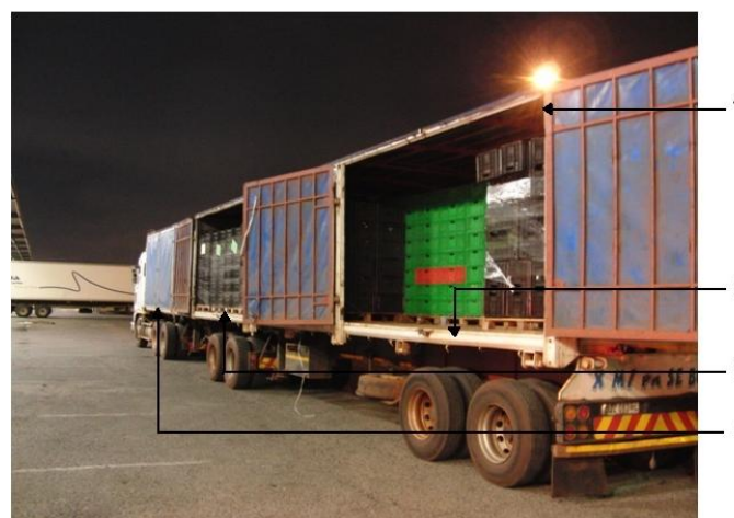
Figure 2: Position of accelerometers on trucks.
