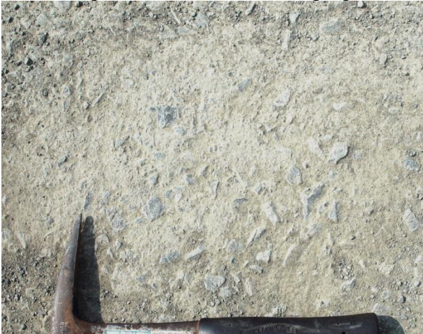
Photo 3: “Gravel-compacted” G1 material.
