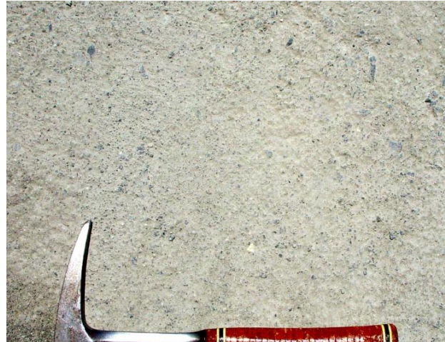
Photo 4: “Water-roll compacted” G1 material.
