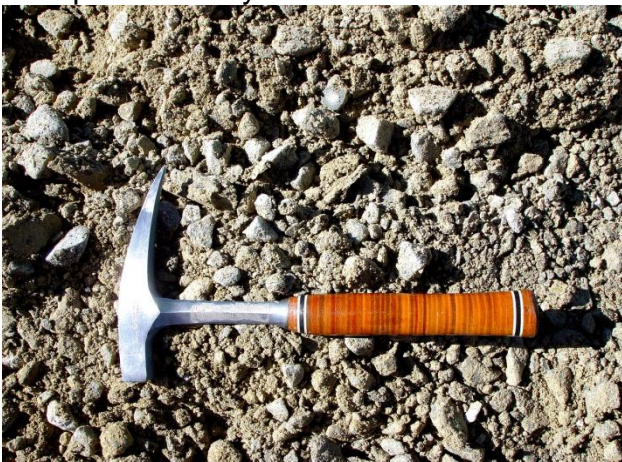
Photo 1: Loose G1 material.
