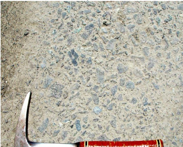
Photo 5: “Slush-compacted” G1 material.
