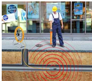
Figure 13 – EasyLoc in operation (My Pipe Lines, 2009)
