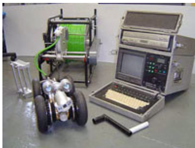
Figure 2 – Crawler drain camera system (My Pipe Lines, 2009)
