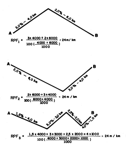
Figure 3.1 - CALCULATION OF RISE PLUS FALL FOR DIFFERENT VERTICAL PROFILES.
