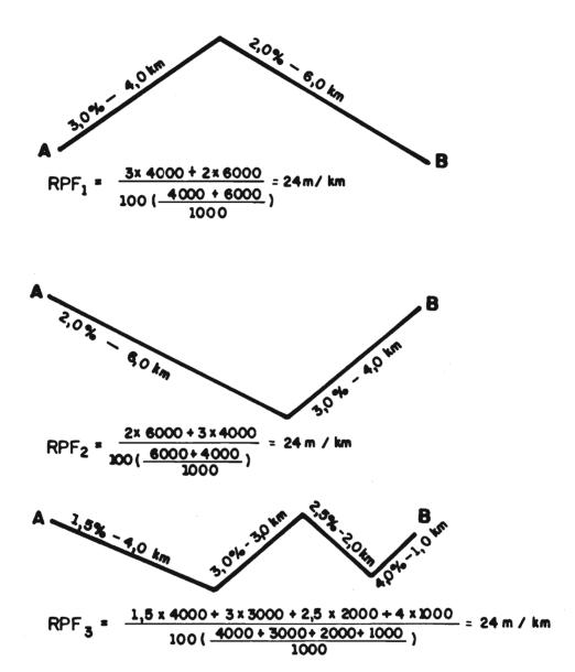
Figura 3.1 - CALCULATION OF RISE PLUS FALL FOR DIFFERENT VERTICAL PROFILES.
