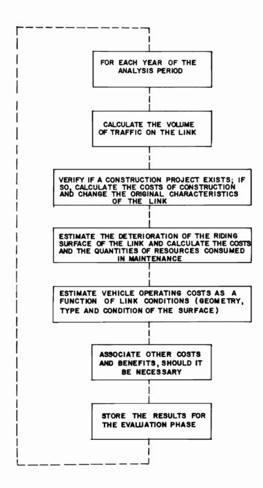
Figure 2.1 - SIMULATION OF A LINK ALTERNATIVE.
