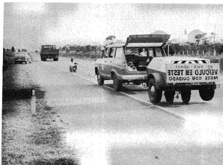
FIGURE 5.4 - DYNAFLECT SENSORS IN POSITION AND READY FOR TESTING
