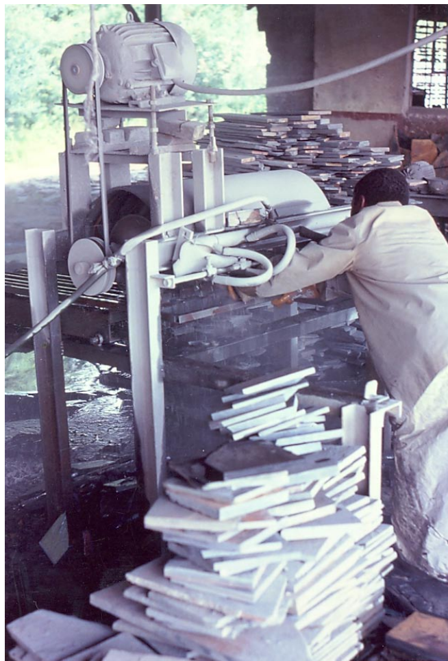
Figure 29 Slate tiles cut to standard sizes with an electric saw (photograph: M. Naudé).
