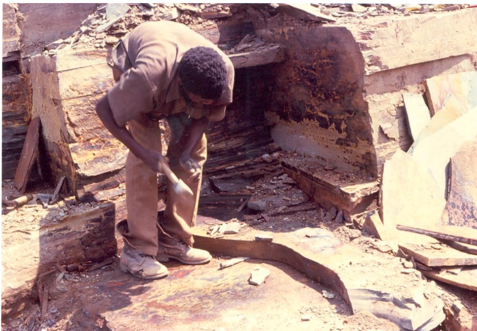
Figure 2 Preparing well-defined profiles prior to inserting the wedges at various places to start the cleaving process (photograph: M. Naudé).
