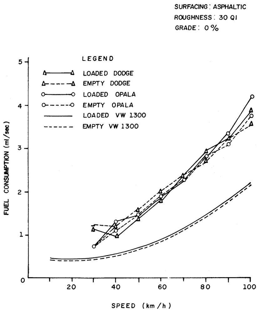
FIGURE 8.5 - FUEL CONSUMPTION OF THE VW 1300, DODGE AND OPALA AS A FUNCTION OF SPEED.
