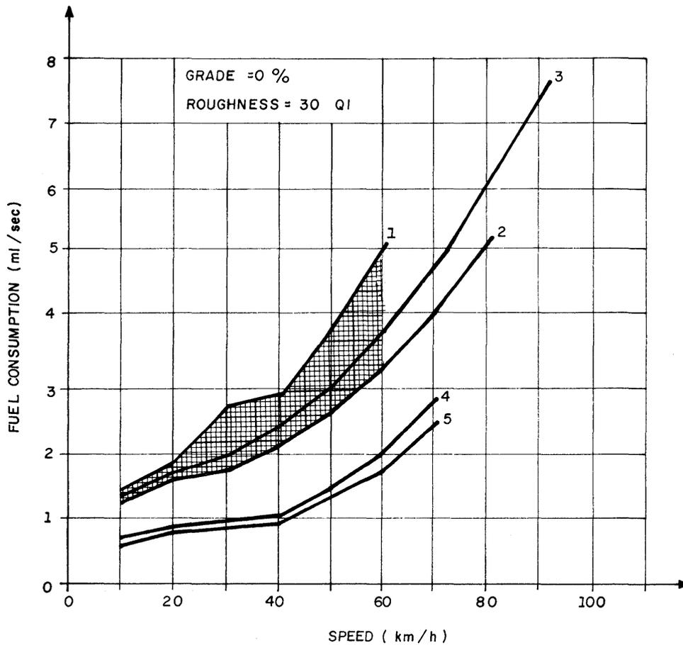
1. Light gasoline truck, empty and using the lowest gear
