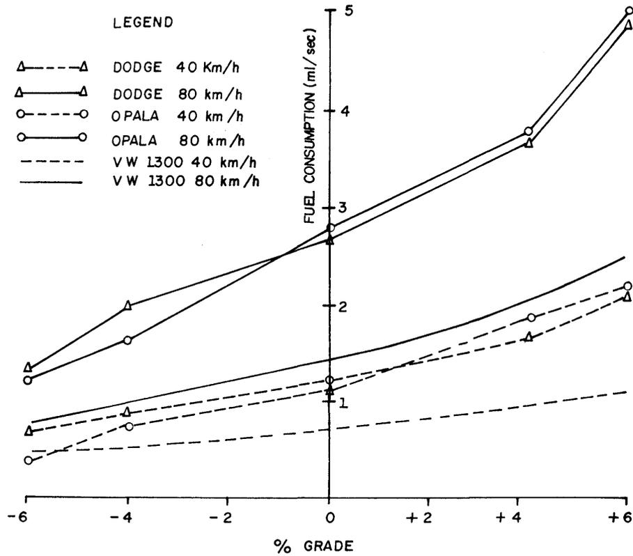
FIGURE 8.6 - FUEL CONSUMPTION OF THE VW 1300, DODGE AND OPALA AS A FUNCTION OF GRADE
