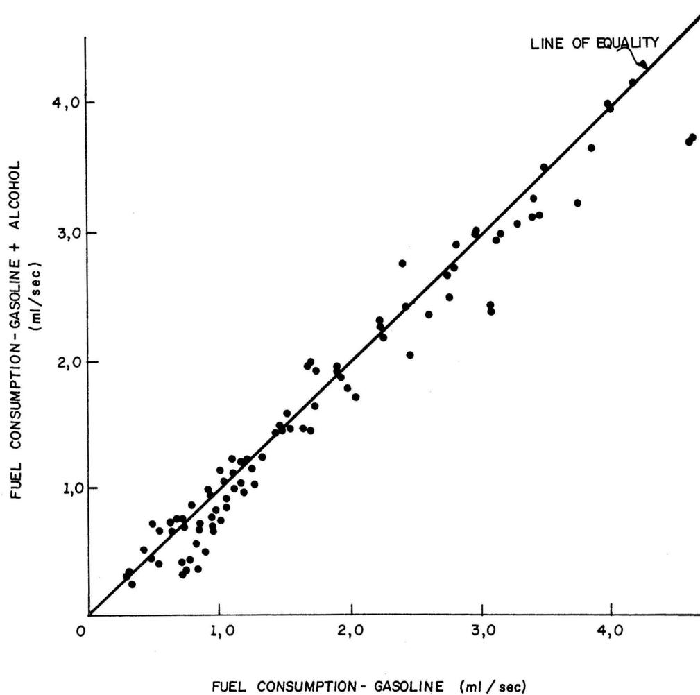
FIGURE 7.3 - GRAPH COMPARING THE CONSUMPTION OF PURE GASOLINE WITH THAT OF GASOLINE + ALCOHOL (UTILITIES).
