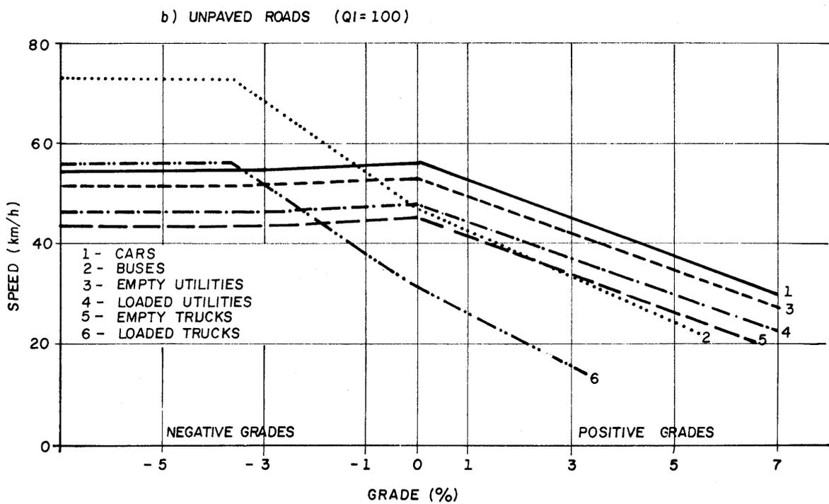
FIGURE 4.1 - VEHICLE PERFORMANCE ON UNIFORM GRADES ( STEADY-STATE SPEED )
