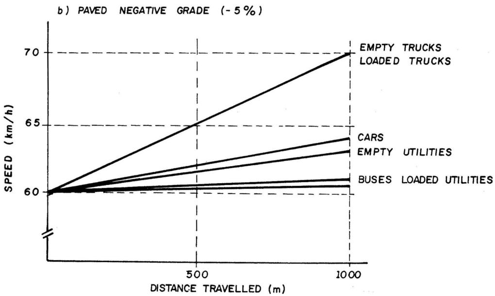
FIGURE 4.2 - VARIATION OF FREE-FLOW SPEED ON CONSTANT GRADES
