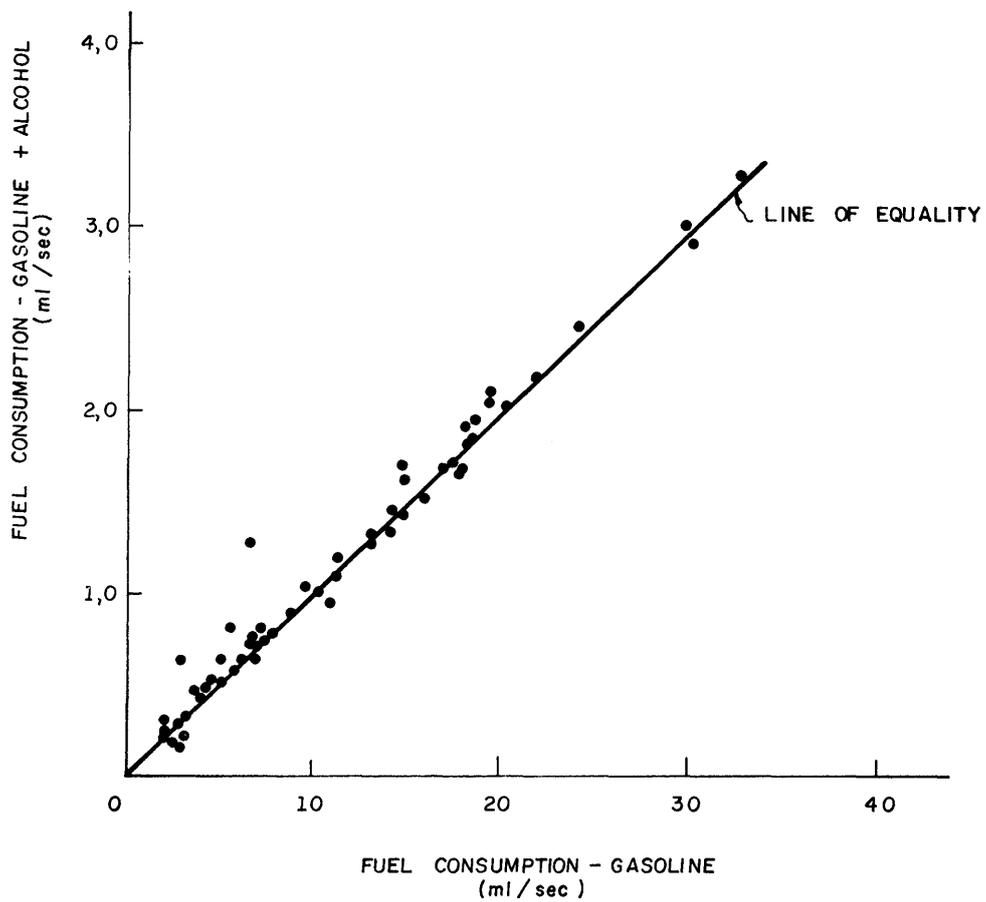
FIGURE 7.2 - GRAPH COMPARING THE CONSUMPTION OF PURE GASOLINE WITH THAT OF GASOLINE + ALCOHOL ( VW - 1300 CAR )
