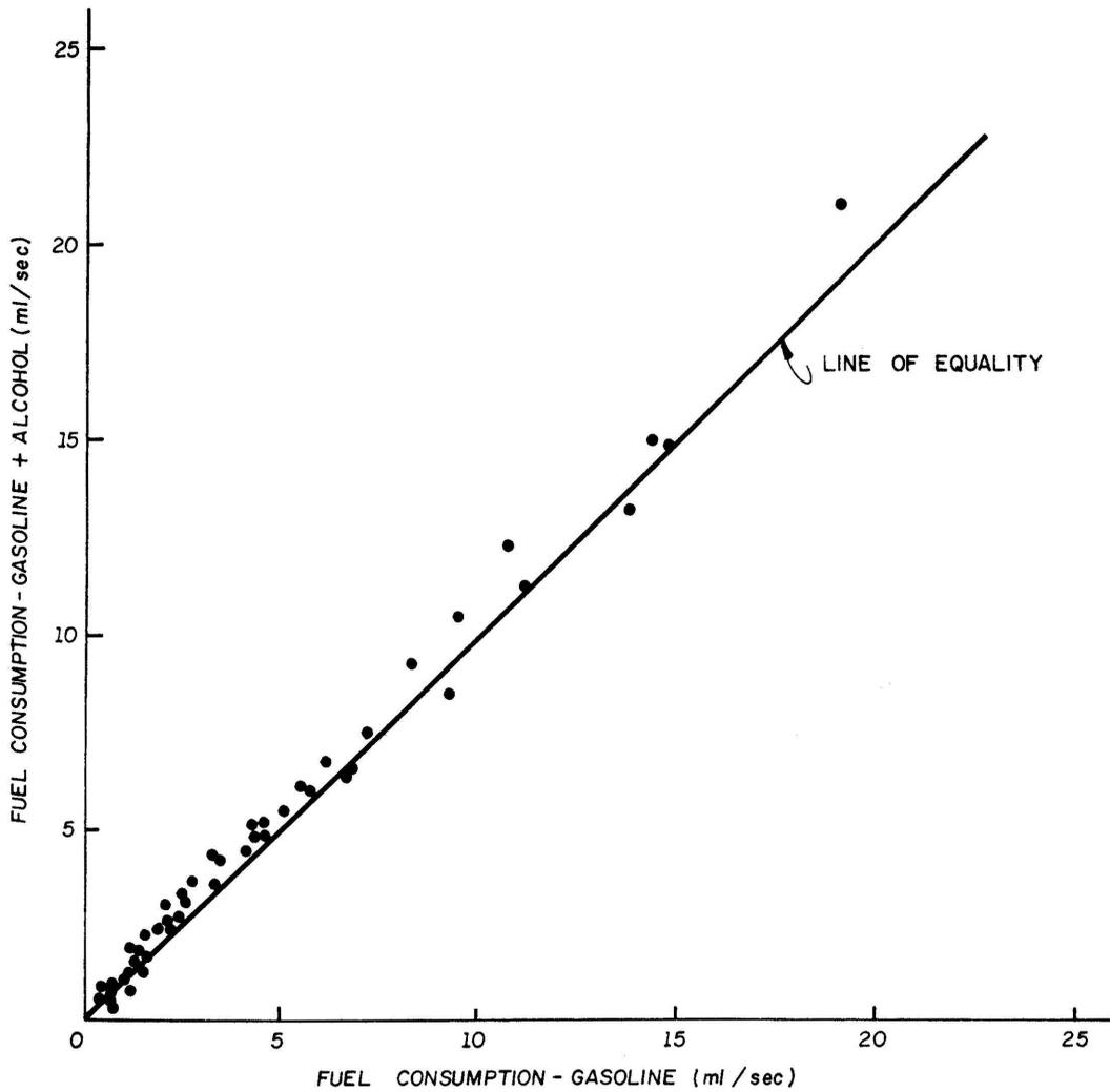
FIGURE 7.1 - GRAPH COMPARING THE CONSUMPTION OF PURE GASOLINE WITH THAT OF GASOLINE + ALCOHOL (LIGHT GASOLINE TRUCK).
