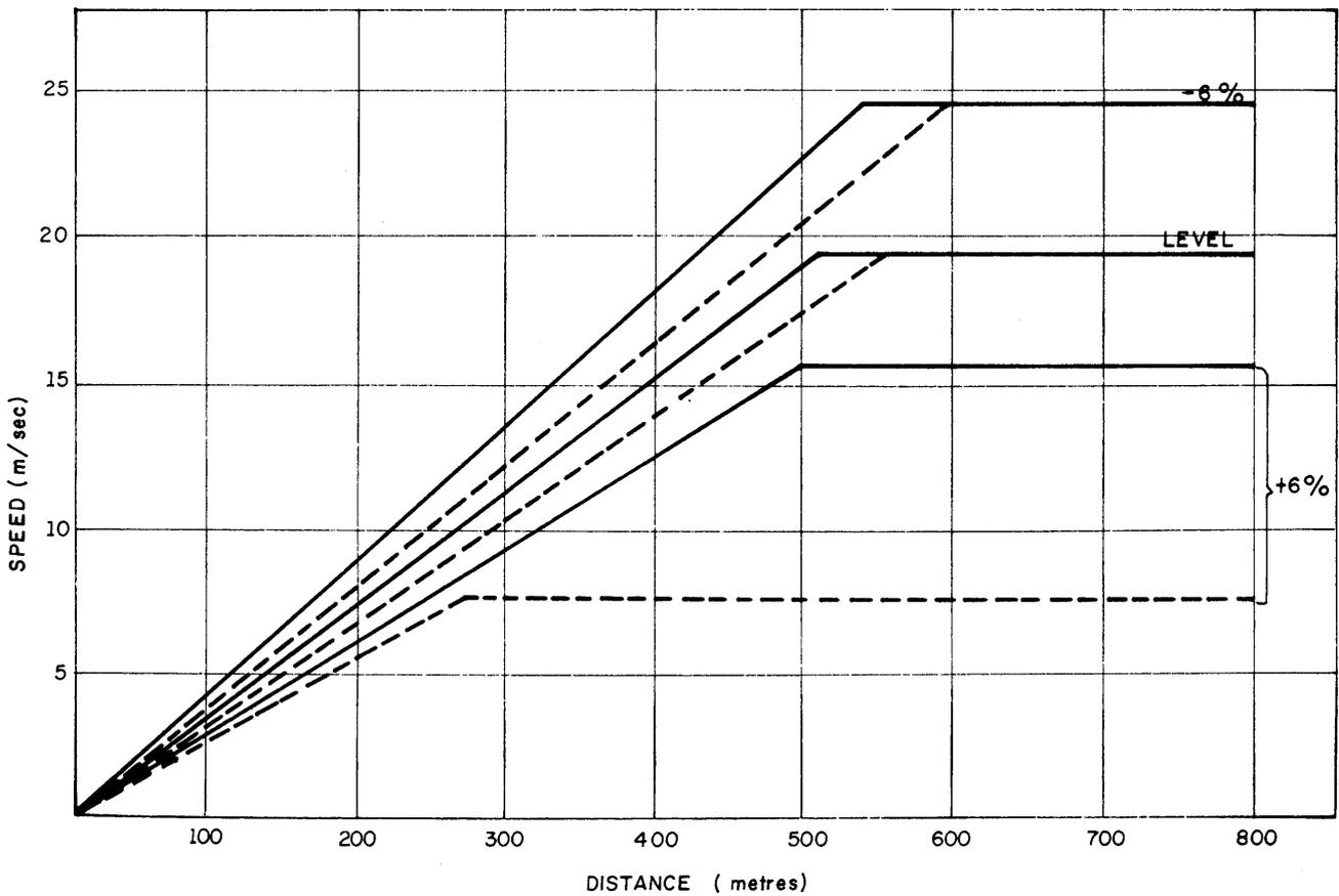
FIGURE 6.1 - CHANGE IN SPEED AS A FUNCTION OF DISTANCE RUN BY VEHICLE
