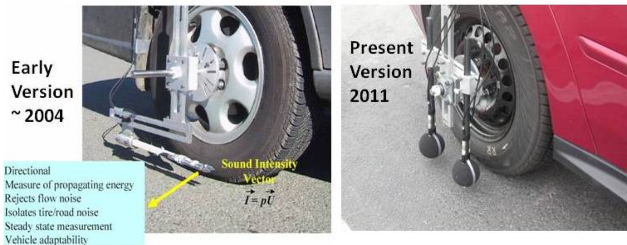
Figure 4. Early version of the OBSI equipment of measuring noise
