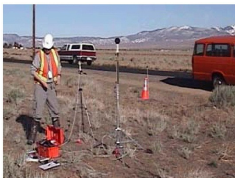
Figure 2. Wayside method of measuring noise
