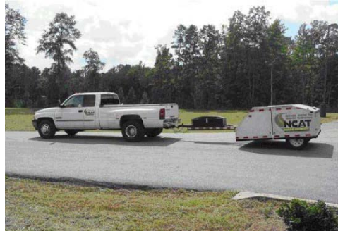
Figure 3. CPX trailer method of measuring noise
