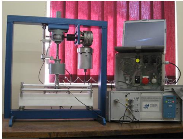
Figure 1: Simple flexural strength determination device
