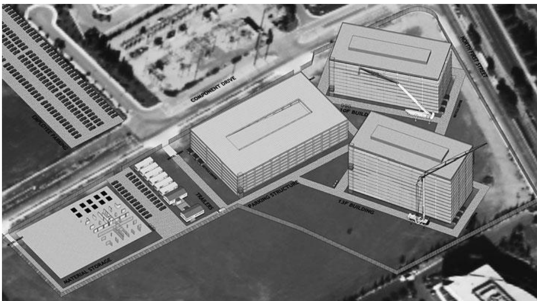
Figure 5: A SketchUP model rendered in Google Earth. Source: Building Information Modeling, Kymmel, 2008
