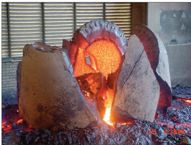
Figure 12—Internal structure of a partially solidified block, as revealed by failure during tipping after primary cooling in the pot
