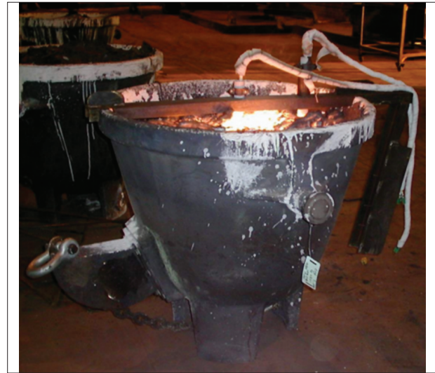
Figure 7—Photograph of a slag block and pot directly after thermocouples were inserted into the block. For support the refractory tubes were inserted into the slag through slots in a steel channel, which was placed horizontally over the pot edge
