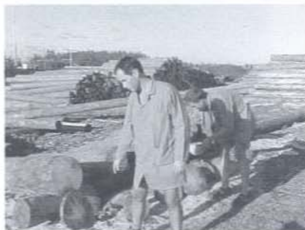
Wilhelm de Beer and Bernard Slippers examining blue stained logs at Richards Bay harbour
