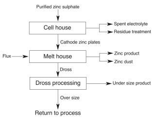
Figure 1—Electrowinning (cell house), melting (melt house) and dross processing stages of Zincor process—after Van Dyk1 and Du Toit2
