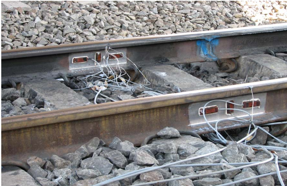
Fig 4. A view of the test site showing the positions of the thermo-couples to measure the spread of heat in the rail profile, and strain gauges to measure forces exerted by the passing train wheels.
