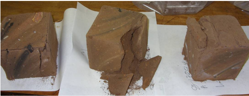
Figure 9: Examples of cubes after UCS testing (triplicate tests on covered N cement cubes)
