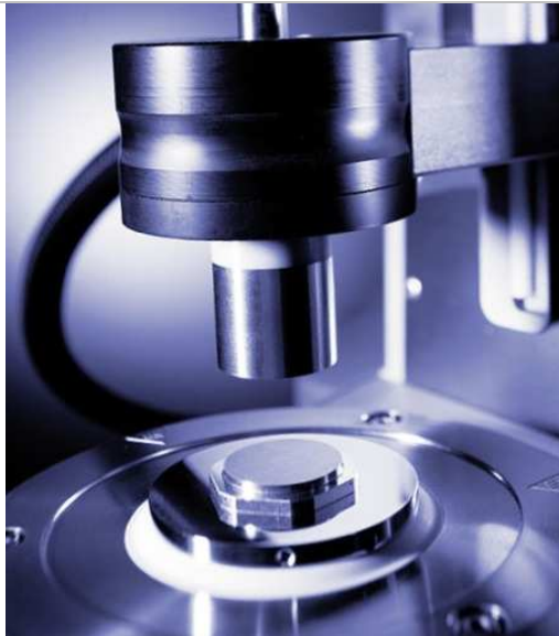
Figure 13: close up of a DSR parallel plate configuration
