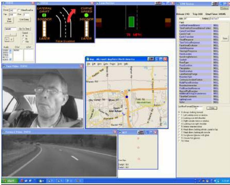
Figure 2: NDS in-vehicle recording instrumentation (Sayer, 2005)
