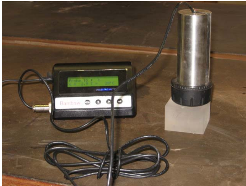
Figure 1: The Rainbow Instruments Dielectric Sensor. Measuring unit, probe with 3lb weight placed on the Perspex block used to regulate the sensor.
