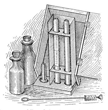
The apparatus delineated above is one devised by Dr. Watkins-Pitchford and named by him the "Isometer". It is used for the estimation of the exact percentages of arsenic present in any sample of dipping fluid. Two tubes, one of which is graduated, are held in a metal frame attached to one end of the containing wooden case. This frame serves as a stand for the testing apparatus which is blackened to prevent reflection of light through the fluids.
