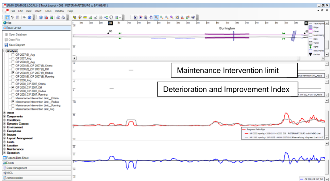
Figure 11: Maintenance Intervention limit compared to Deterioration and Improvement Index
