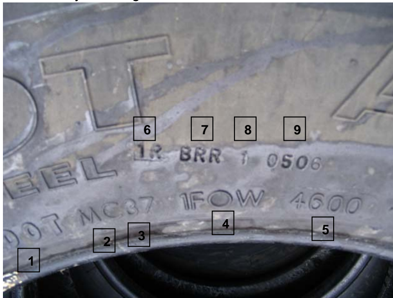
Figure 3 Mandated Tire Identification Marks on a Casing Source: Woodrooffe et al, 2008
