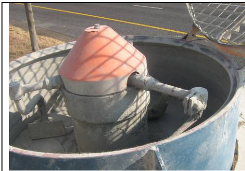
Figure 4: inside of mixer pan
