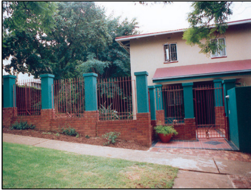
Figure 5: A fence as target hardening measure allows for better surveillance than a solid wall
