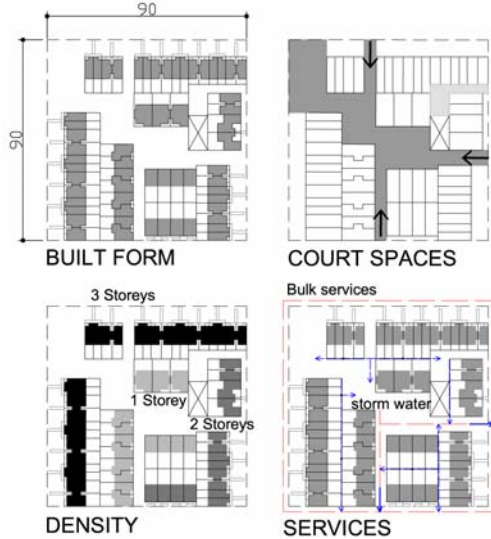
Figure 4: Typical 90m x 90m block
