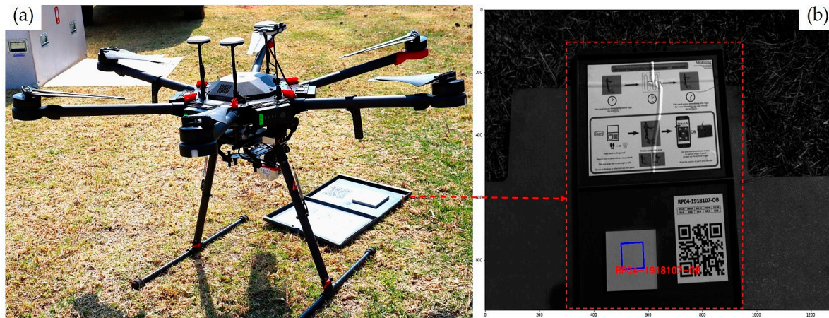
Figure 4. Multi-rotor DJI Matrice 600 Pro system equipped with MicaSense RedEdge-MX sensor (a) and a MicaSense Calibration Reflectance Panel serial number: RP04-1918107-OB (b).
