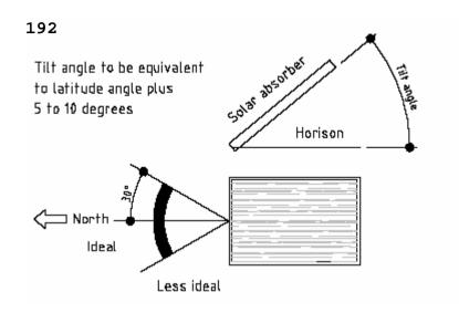
To raise the temperature of 200 litres water by  $43^{\circ}\text{C}$  (as typically consumed by a family of four per day) one needs 10kWhr of energy20. A typical (200 litre) hot water storage tank may need to warm water from  $17^{\circ}\text{C}$  to  $60^{\circ}\text{C}$ . Water has a high specific heat (C) of 4200J/kgK and a density of 1kg/litre.
