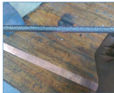
Fig. 1 Nickel foam placement in the open rectangular channel
