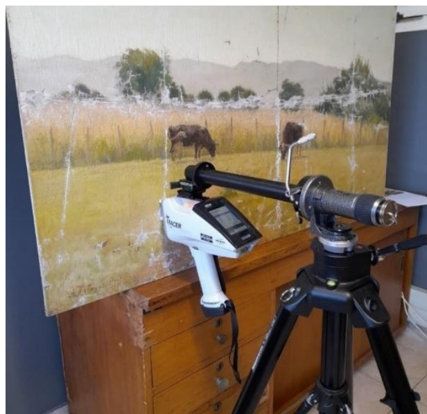
Figure 20: XRF set-up for analyses on Cattle Grazing near Pretoria Zoo (c 1896). Van Wouw House, Pretoria. Photograph by JA Elsenbroek.
