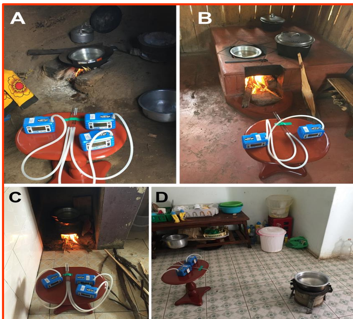
Figure 3. Typical sampling setup used at (A) Narok rural HH#1 (Improved 3-stone) (B) Bomet rural HH#1 (Improved 3-stone) (C) Bomet urban HH#1 (Jiko), and (D) Narok urban HH#2 (Jiko). For all samples, the PDMS trap was positioned at 65 cm from the stove and at a height of 36 cm above the ground.
